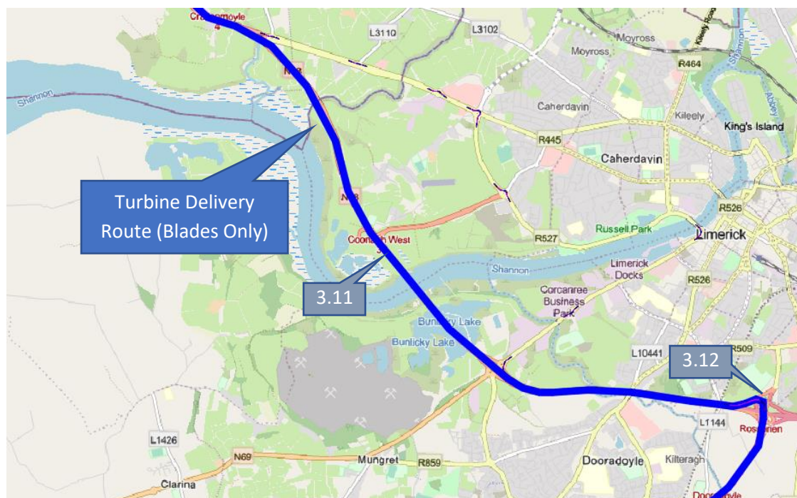
Figure 3 – Turbine Delivery Route Pinch Points (Limerick)
