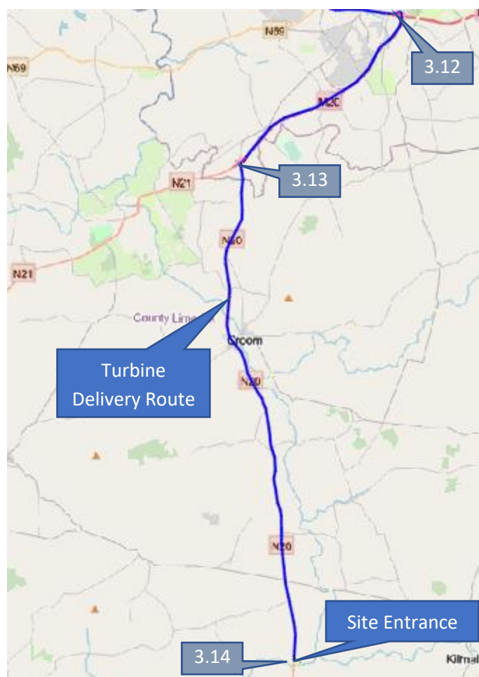
Figure 3 – Turbine Delivery Route Pinch Points (Limerick)
